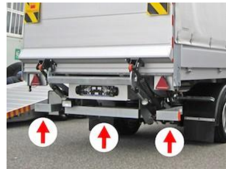
Fixed 3-piece bumper in steel, mounted to the lift frame
